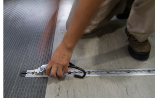
MTM Transit operator adjusts wheelchair securement belts.
