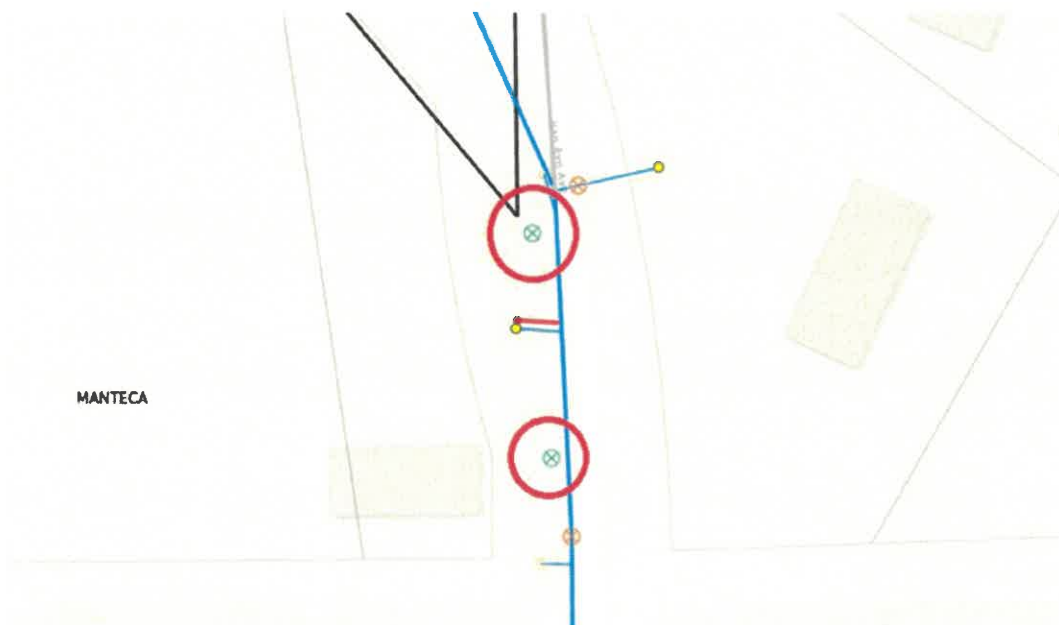
Missing Features: Floating Valves – likely service valves
