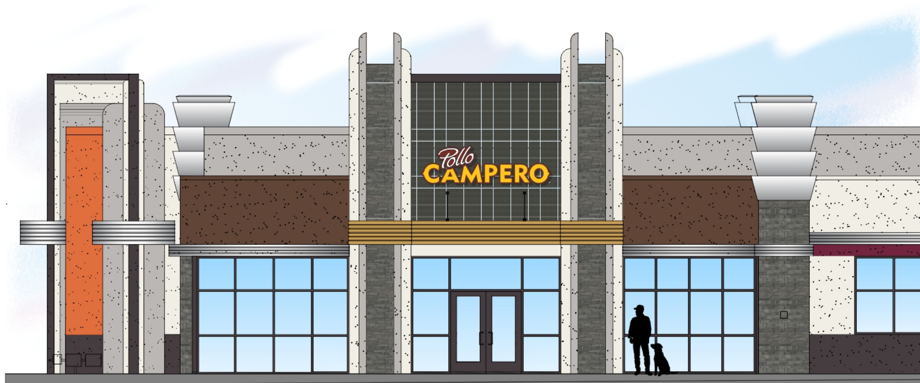
SIGN L / POLLO CAMPEROS SECTION OF BUILDING / EAST ELEVATION / NTS 0.125" = 1'-0"
