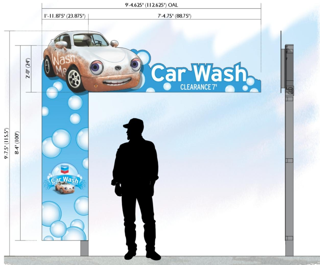
**SIGN D / SINGLE FACED NON ILLUMINATED CAR WASH HEIGHT DETECTOR DISPLAY** QUANTITY (1)
