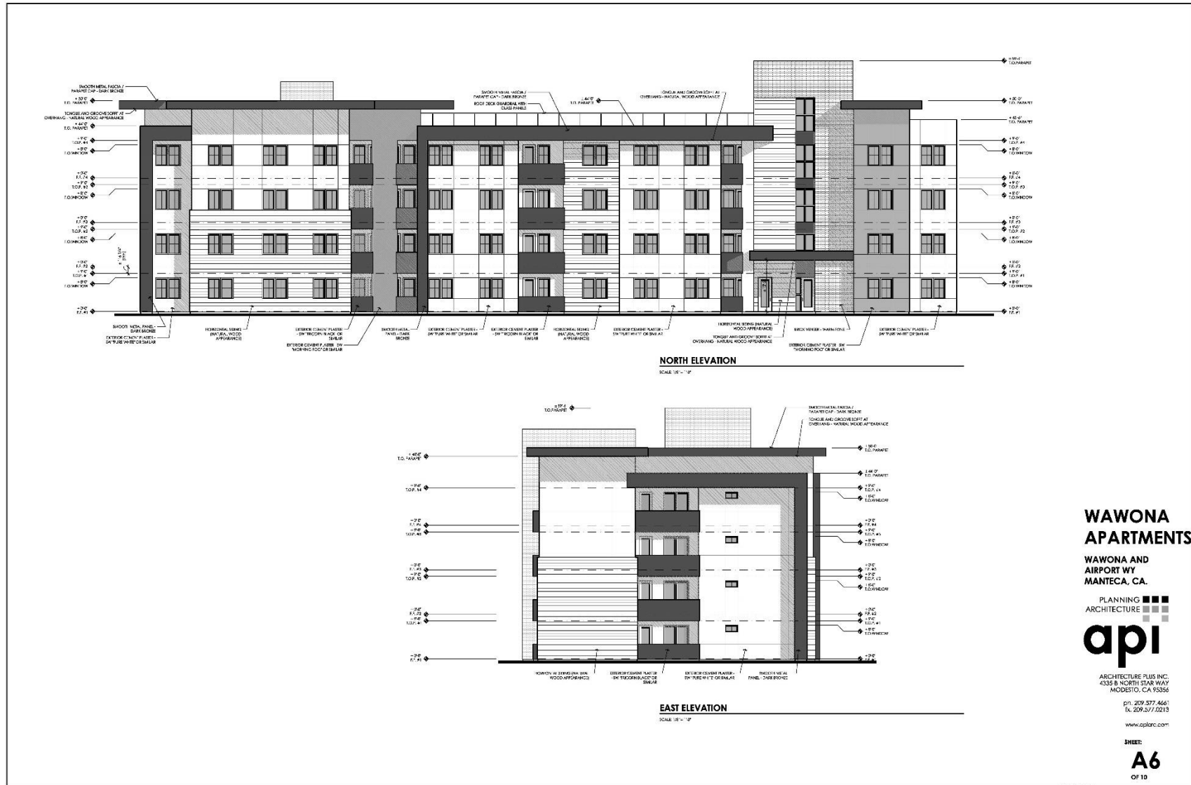
Figure 2-11 North and East Elevations
